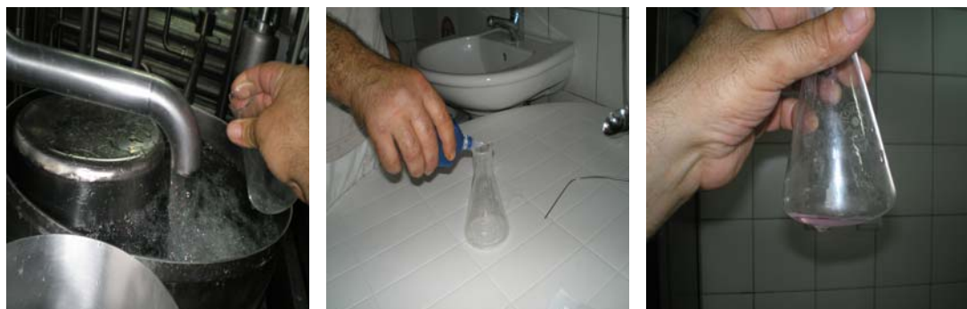
Photo 2 Verification of purification of the process by the method of phenolphthalein as an indicator
